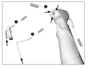
Cleaning of the external coolant tubes Cleaning of the spray nozzles with WS-91 L G, WS-91. WS-92 L G. WS-92
