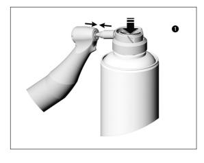
WS-91 L G, WS-91, WS-92 L G, WS-92 Weekly oil service of the chucking system
