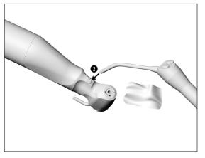
2 Blow the LED dry with air syringe or dry it carefully with a soft cloth.
